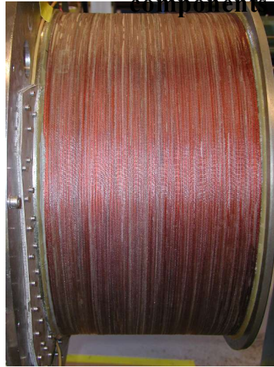
Main (trapezoidal) coil: from first to last (64 th ) layer
